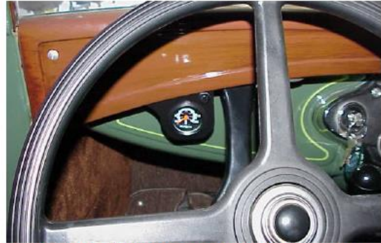
A 1½-inch SunPro mechanical temperature gauge is installed with a custom made bracket up under the dash rail of a 1931 Victoria.
